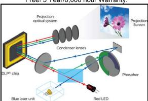
By combining a laser, a fluorescent element and an LED Casio has created an original mercury-free hybrid light source capable of generating high brightness. Casio has achieved high brightness output of green light, which until now, has been considered difficult with conventional semiconductor light sources, by efficiently converting blue laser light into green light using a fluorescent element.
