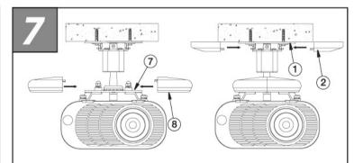
To complete installation attach the two halves of the carousel coverplates (part 8) over the carousel disc (part 7), then attach the two ceiling coverplates (part 2) over the ceiling bracket (part 1).
