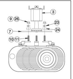
Insert M4 allen screw (part 5) into the top of ball-joint bracket (part 3).
