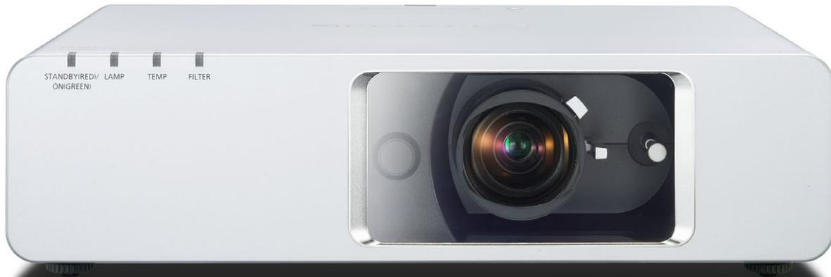
In addition to being bright and easy to use, the PT-F300 Series LCD projectors give you enhanced performance with minimal maintenance over time. Highly reliable optical block and a long operating life are ensured by the use of inorganic materials for the LCD panels and polarizers. The new Auto Cleaning Filter (ACF) extends the filter replacement cycle to over 10,000 hours,\*<sup>1</sup> and together with the dust-resistant design boost reliability.
